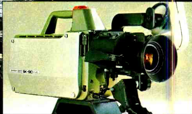
Hitachi SK-90: portable ENG mode
