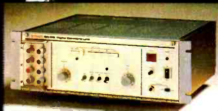
Digital Command Unit (with coax/triax option)
